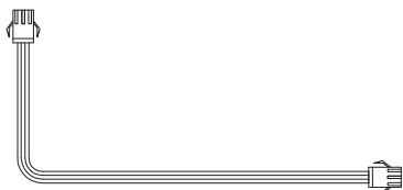
F3. 3 PIN Tension Knob Connect Wire x 550m/m
